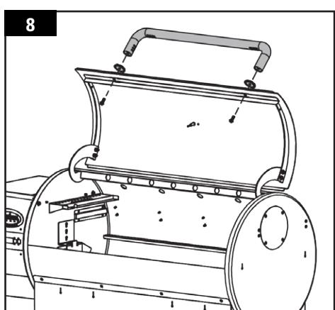
**NOTE: Do not over-tighten screws. Only a snug fit is necessary.**
